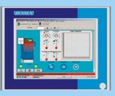
Easy operation of the dryer control over Panel-PC with touch screen.
