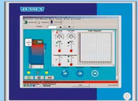
Easy operation of the dryer control over Panel-PC with touch screen.
