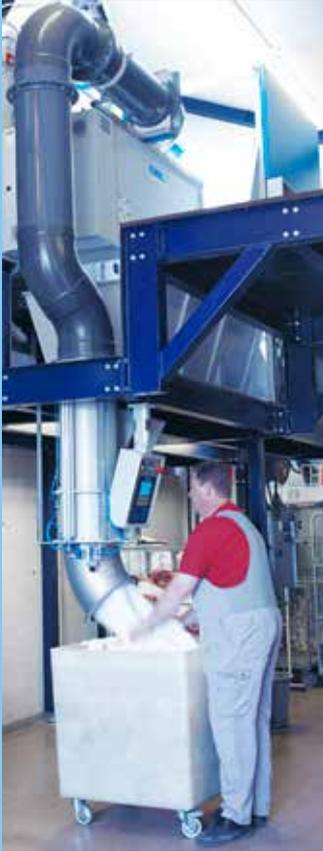
Vacuum loading through the unloading door of the dryer with the VacuTrans system
